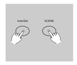
2. Press and hold down the Auto/Del button. While holding down the Auto/Del button, tap the Scene button that stores the scene you wish to delete.
