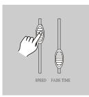
After selecting the bank of scenes you wish to run, you can use the Speed slider(or Tap Sync/ Display button) and Fade Time slider to adjust the scenes to your desired effect.
