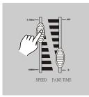
3. Use the Speed slider(or Tap Sync) and Fade Time slider to adjust the chase to your desired effects.
