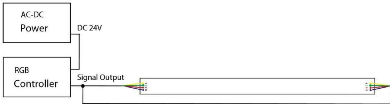
Type 2. Single Power Supply, Double Ends Feed
